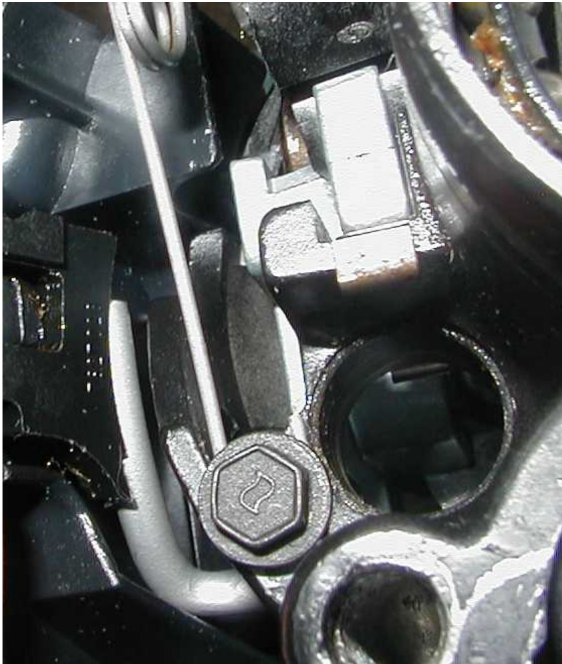
Tilt lever housing seated against column, note how the follower is oriented:
