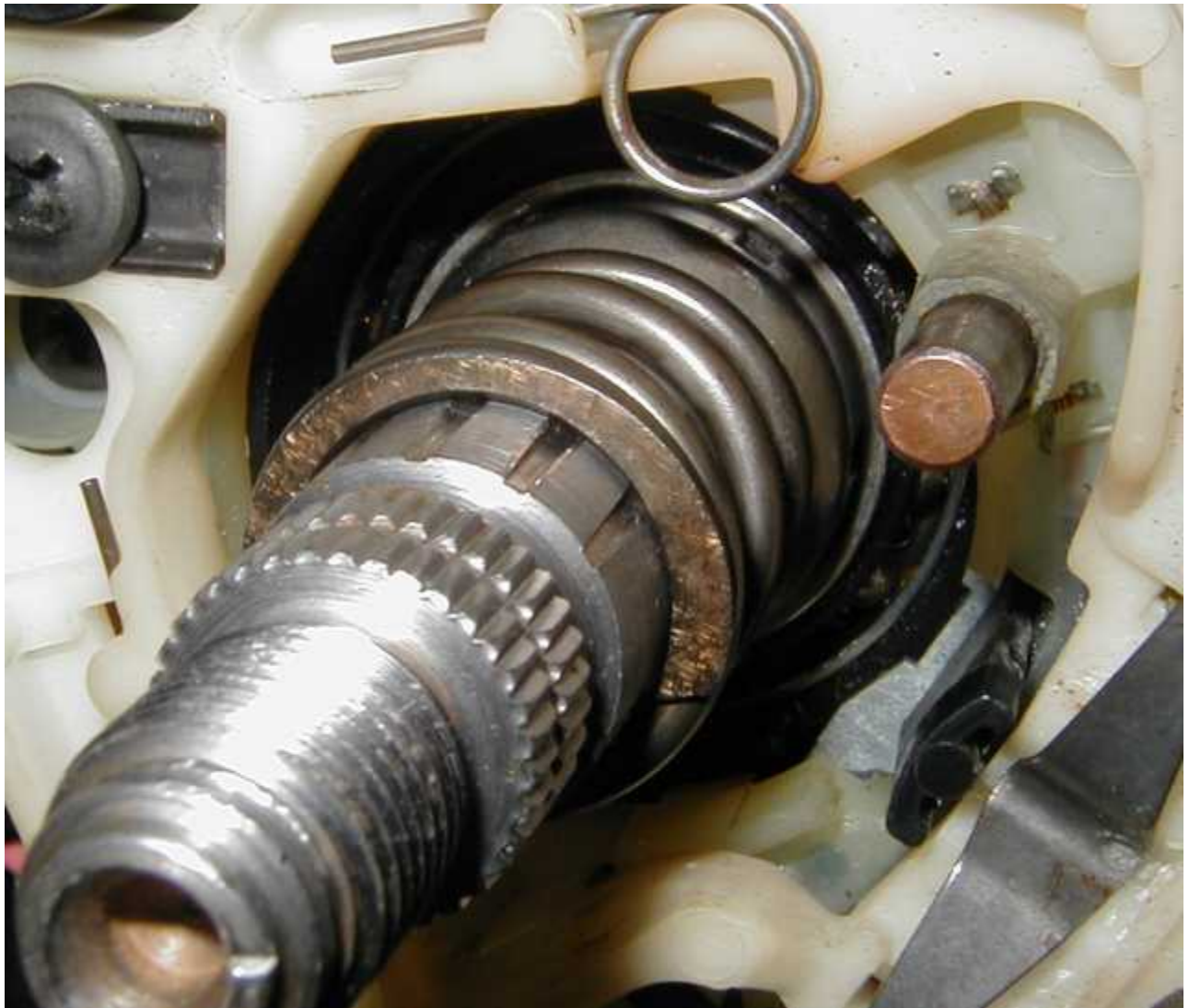
A top view of the cancel cam, the tube sticking up holds the horn button contactor:
