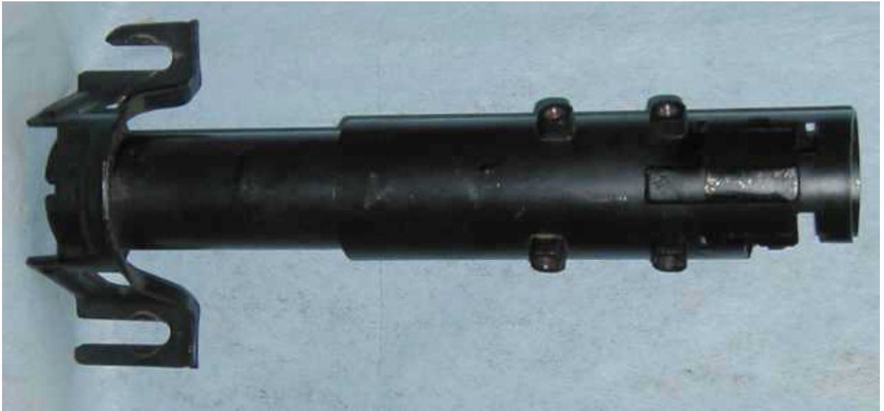
This is the lower bearing with dust shield and ( 2 ) 8-32 x 1" self-tapping deformed-thread screws:
