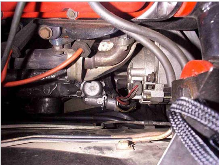
Governor housing is located below alternator
