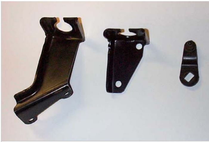
(L to R) Stock bracket, modified bracket, and shift lever
