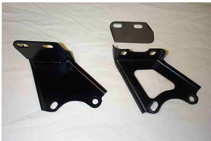
Transmission to engine mount (for 3.4 L)
