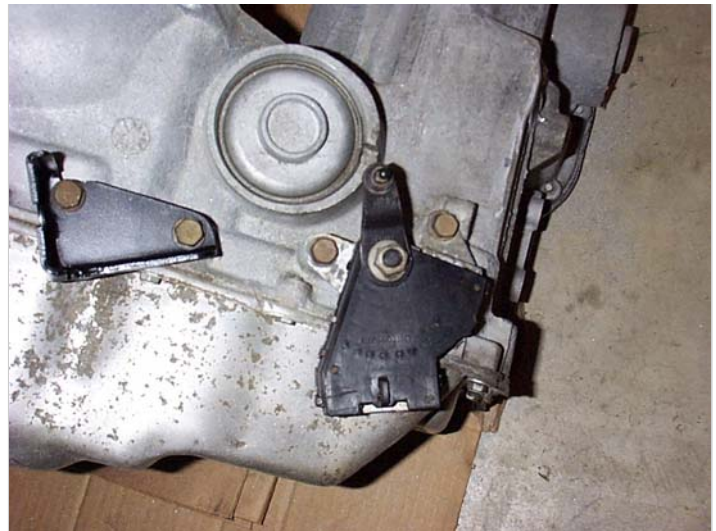
Bracket on transmission with shift lever in neutral
