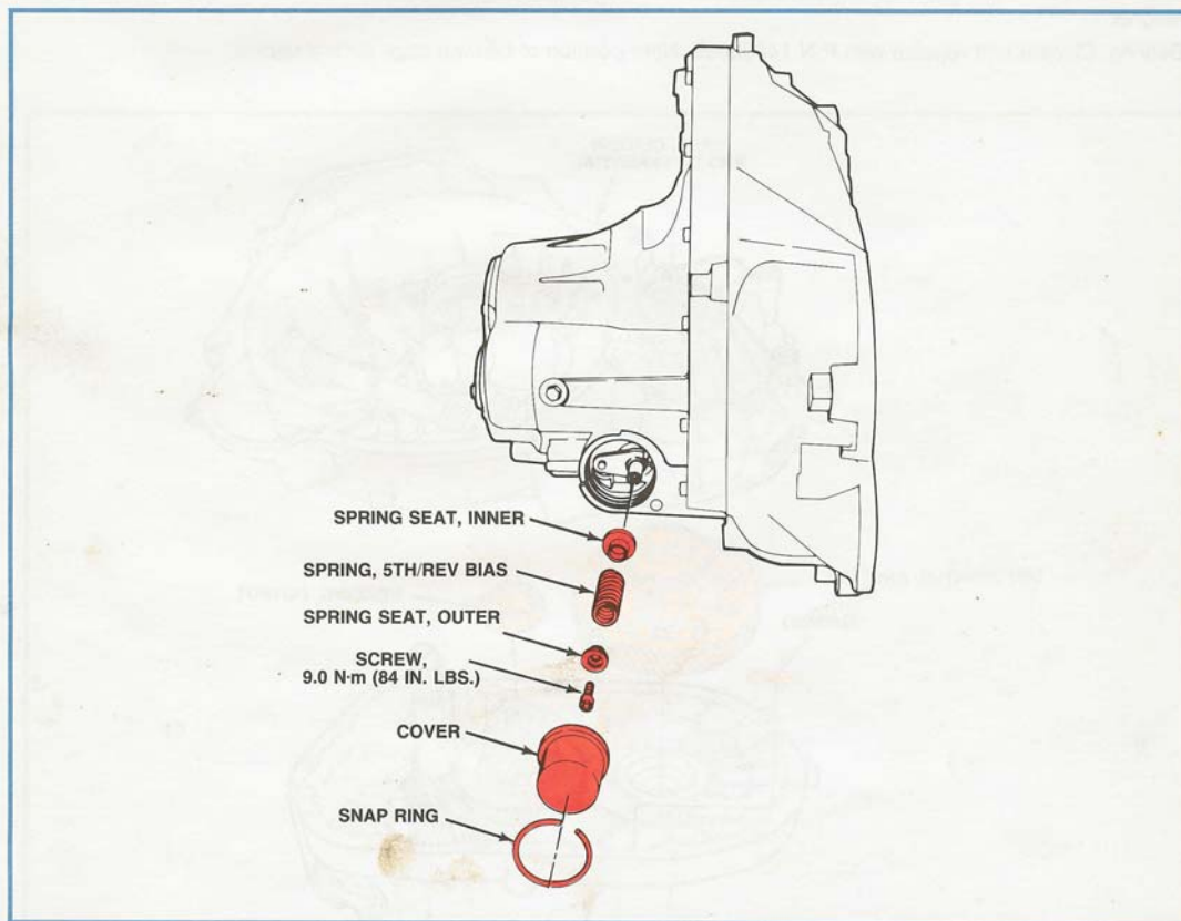
Figure 5-3, Shift Shaft Detent Components/Transmission Housing.
