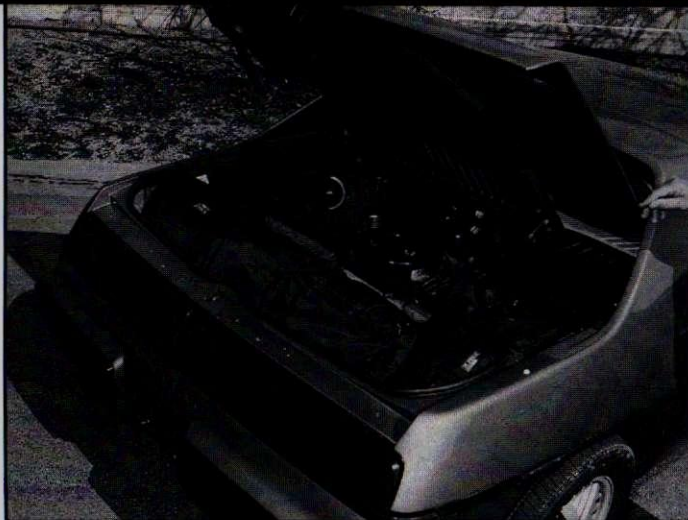
For 1984 only, Fiero's engine cover grille was cast magnesium. Two golfbags or 5 upright sacks of groceries fit into the 5.65-cu.-ft. rear storage compartment.
