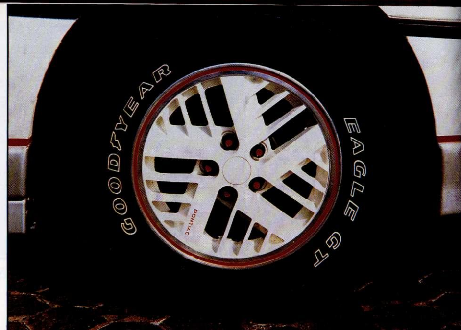
Pace Cars' standard Hi-Tech Turbo alloy wheels were painted white, with red lug nuts and trim. Tires were P215/R60-14 Goodyear Eagle GTs.
