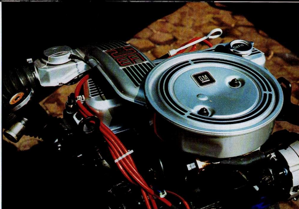
All 1984 Indy Pace Car replicas used the Fiero's 92-bhp Four, retrimmed with special graphics, silver aircleaner and rocker cover, plus red ignition wires.
