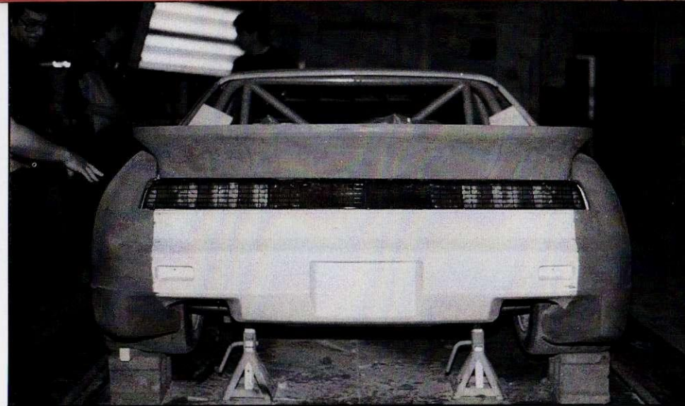
GM modelers apply clay over an actual DGP Stage II body to create Stage III. Female molds are taken from the clay, then fiberglass gets laid up inside molds.
