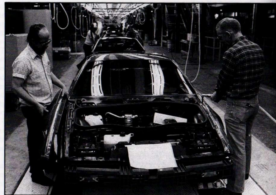
Enduraflex panels, painted in matching sets, are installed near end of assembly line. Car is then checked for leaks before interior goes in.
