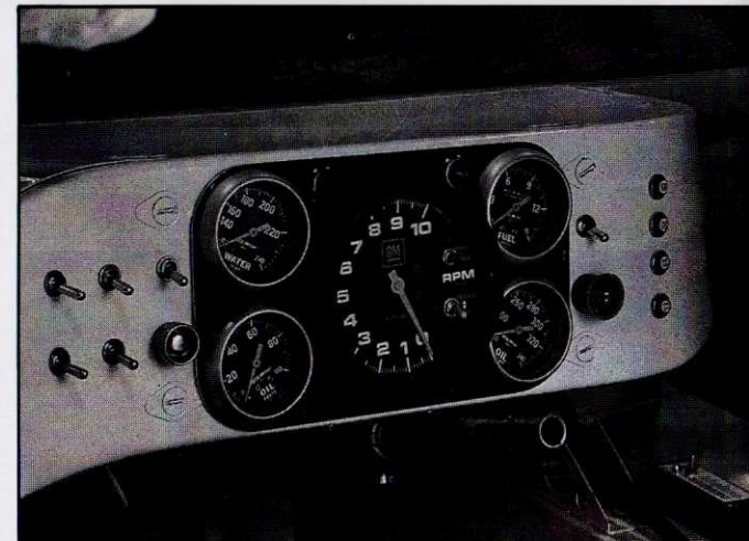
Fiero GTU's no-nonsense interior houses 29-gallon fuel cell inside aluminum center console. Ten-grand tach dominates instrument cluster. All needles point straight up if everything's normal.
