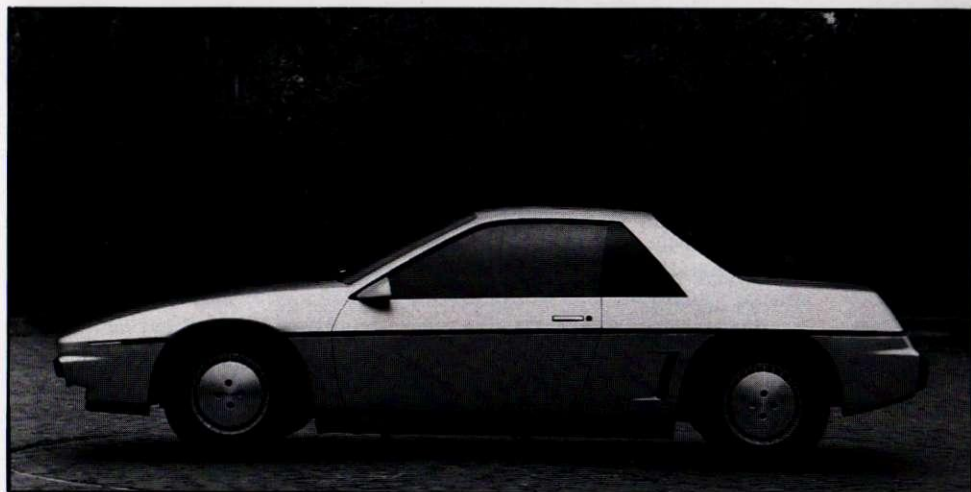
It soon became necessary to widen B-pillar to accommodate space frame's rollbar as Hill's group explored variations on their original theme.
