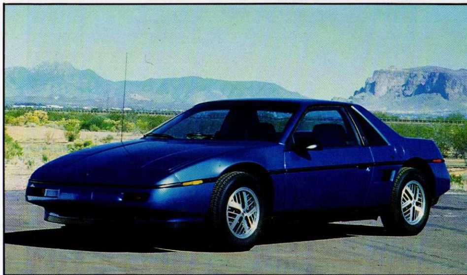
Blue-for-1987 Fiero Sport Coupe shows off restyled front end, without black bumper pads. Plastic body skins make facelifts easy and relatively inexpensive.
