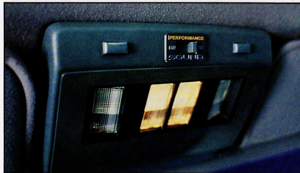
The 1986-87 Fiero's overhead console incorporates twin map lights, dome light, and a slide switch to alter the intensity of the Performance Sound system.
