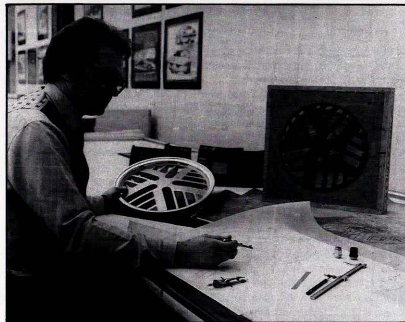
General Motors Design Staff engineer Richard Schell checks mold and early casting for Fiero's 1984 optional Hi-Tech Turbo alloy wheel.
