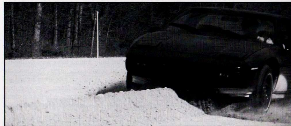
Prototype testing included running over manmade ridges to see if car would ingest dirt. Unpainted black body panels came straight from the mold.
