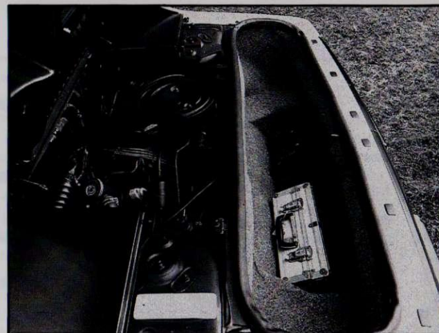
For 1984 only, Fiero's engine cover grille was cast magnesium. Two golfbags or 5 upright sacks of groceries fit into the 5.65-cu.-ft. rear storage compartment.
