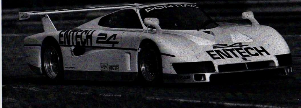
Fiero GTP has a bonded aluminum honeycomb chassis beneath Kevlar skins and uses carbon fiber for the complex front tub. Its 3.0-liter engine delivers 330 bhp.
