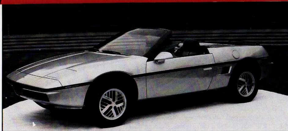
Another engineering experiment, this convertible boasts a folding hardtop that telescopes into itself and stows beneath a section of the rear deck. GM holds
