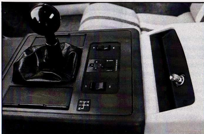
Lighter plus controls for optional window lifts and electric outside mirrors rest in console.
