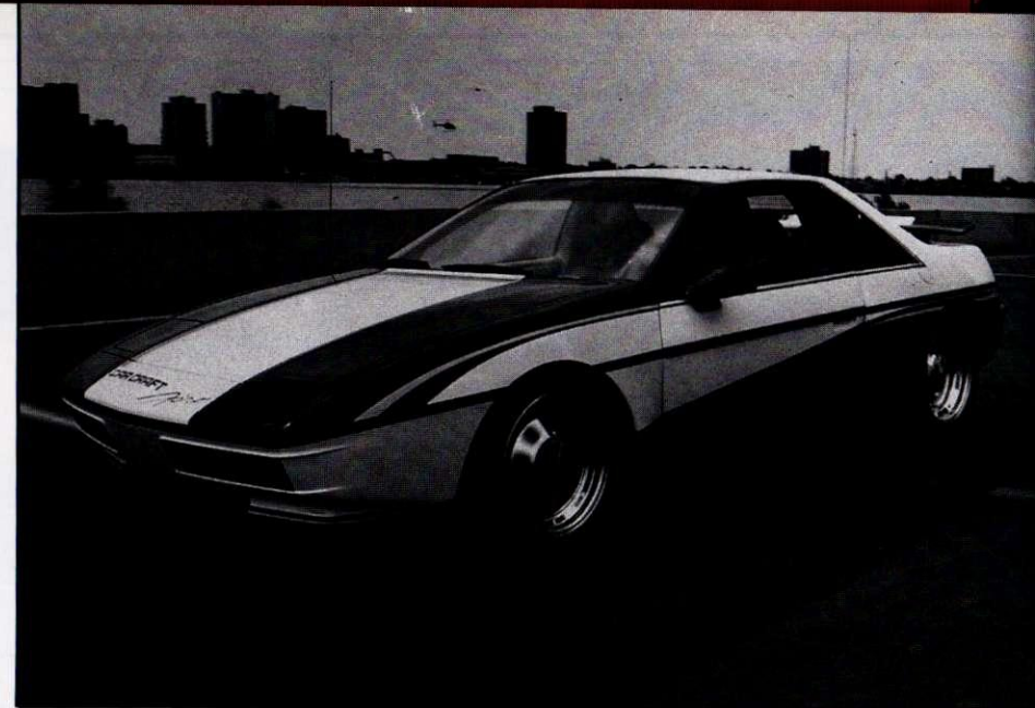
CC's project Fiero used Super Duty engine parts and Herb Adams VSE suspension. Its styling treatment led directly to DGP's Stage II fiberglass competition body.
