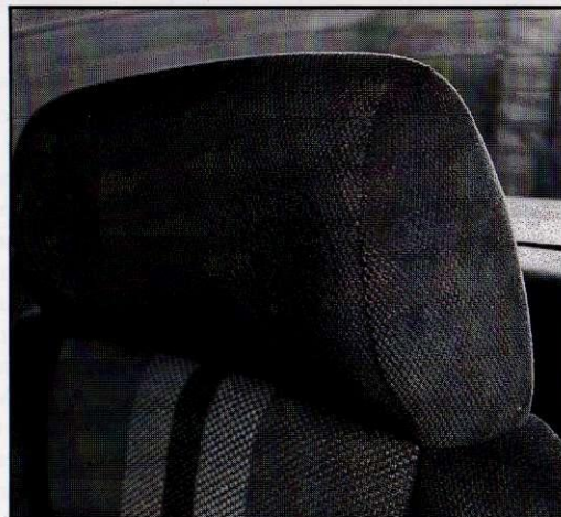
All 1984 Fieros with optional stereo systems came with twin 3-inch speakers in both headrests.
