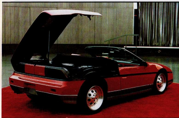
A second convertible was designed and built by Pontiac Engineering to test the side-opening rear deck.
