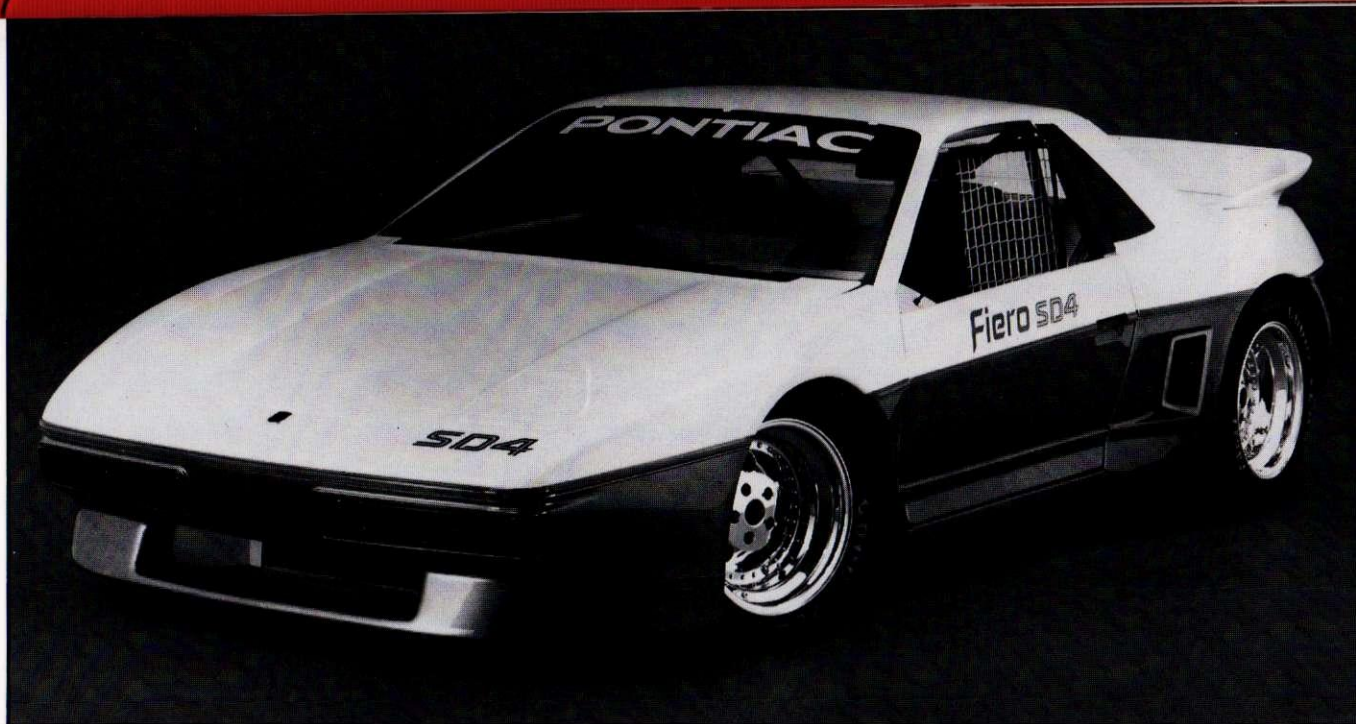
As the basis for most Fiero competition cars that followed, prototype SD-4 made its press debut in June 1983. Tube frame was built in three sections and covered by
