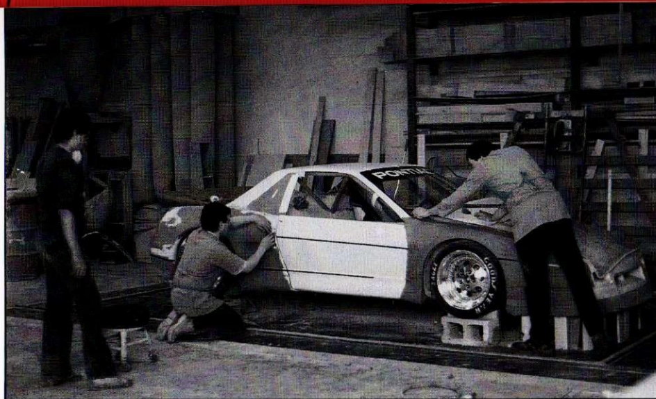
GM modelers apply clay over an actual DGP Stage II body to create Stage III. Female molds are taken from the clay, then fiberglass gets laid up inside molds.
