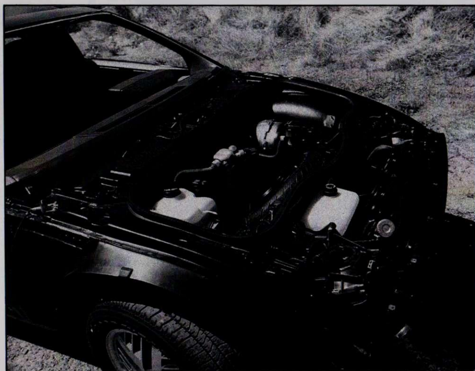
Mini-spare wheel was initially supposed to be aluminum, but production Fieros got a steel version instead. Spare and receiver/dryer leave front trunk tight for space.
