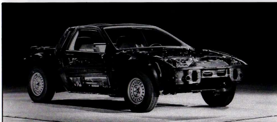
During production, space frame and powertrain become a driveable chassis, which needs no conveyor during the last part of its assembly process.
