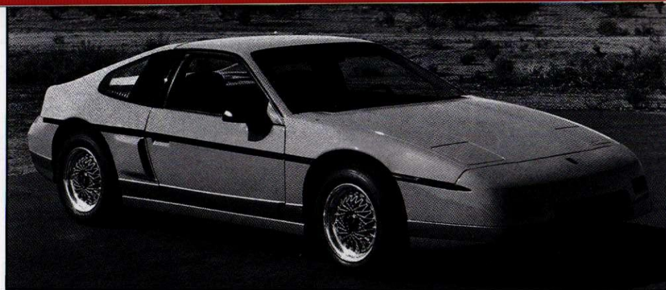
This is the yellow fastback prototype that Jay Wetzel and John Schinella ran by management at Mesa in Feb. 1984. While the body style got overwhelming approval, its experimental, vertical air intakes were shelved due to chipping and clogging.
