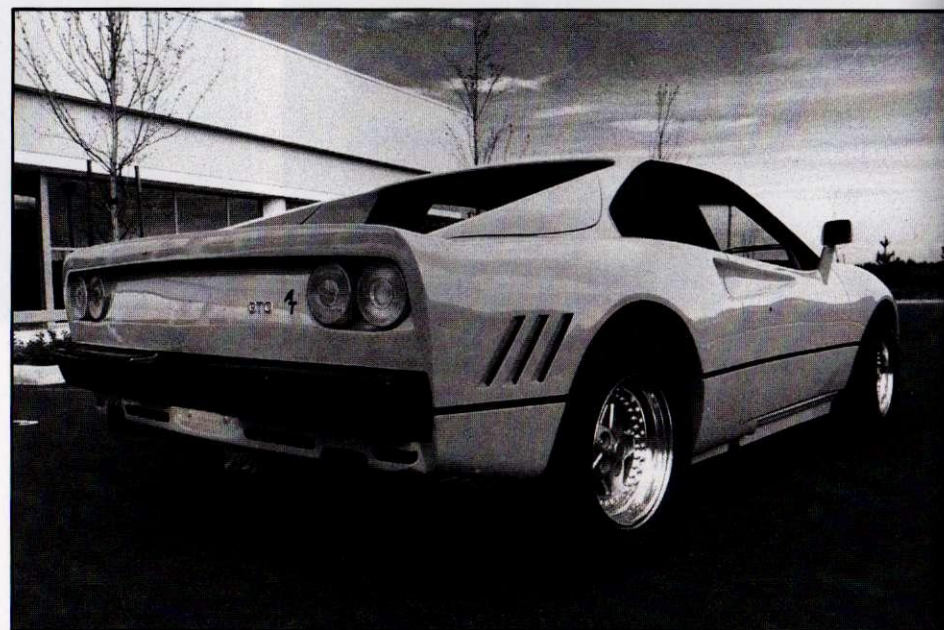
by Alden Thomas in Oregon. All body panels bolt directly to the stock mounting points and require no bonding or fiberglassing.
