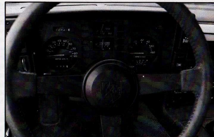
Calibrated in both mph and kph, '84 Fiero's speedo tops out at 85 mph. Tach contains voltmeter.
