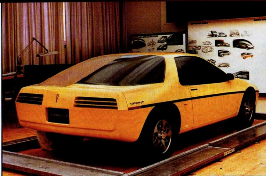
As early as Dec. 1979, Pontiac considered a true fastback "Sprint." Despite good aerodynamics, engine heat retention scotched this design.
