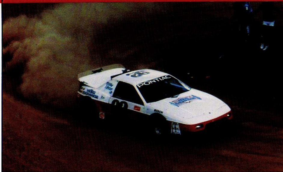
Bobby Unser Jr. storms up Pikes Peak in the 1985 Predator Hillclimb. His car carried stock Fiero body panels over a full Wells Coyote single-seater chassis.
