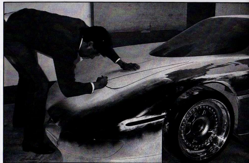
Going by Cafaro’s model, Spice Engineering in England scaled up the GTP full size. Cafaro, seen penning in the air outlets, went to England twice.
