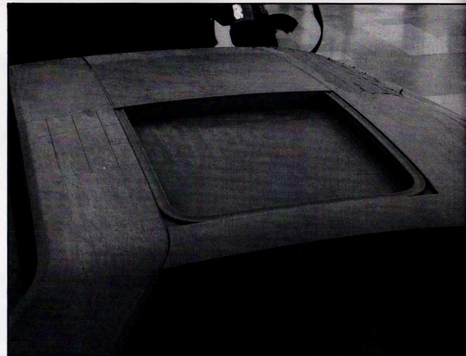
Proposal for Fiero's lift-off sunroof split it in two parts for easier removal and storage. Car's structure wouldn't allow a factory T-top.
