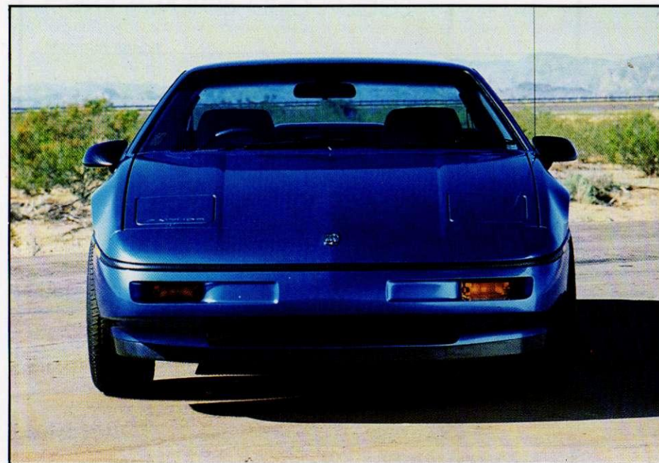
Base 1987 Fiero takes in cooling air under nose. All series except SE get a smooth, convex rub strip, while SE's consists of a 2-channel ribbed molding.
