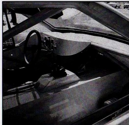
Fiero GTU's no-nonsense interior houses 29-gallon fuel cell inside aluminum center console. Ten-grand tach dominates instrument cluster. All needles point straight up if everything's normal.
