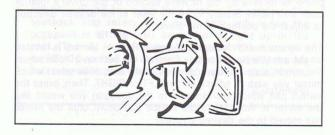
The mirror can be adjusted up, down or sideways to obtain the best view. Move the mirror lever to the night position to reduce glare from the headlights of vehicles behind you.
